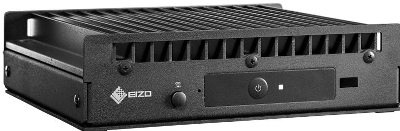
The IP decoder box from EIZO is an integrated solution that can be connected directly to a switch for the connection with IP cameras. Neither a computer nor a software program are required for operation, which makes installation significantly easier and also saves time and effort. Sources of errors and risks for sensitive data, which can result from a traditional configuration with significantly more hardware and software, are also eliminated.
