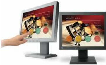
are equipped with an analog resistive touch panel which offers a fast touch response, long touch life, low energy consumption, and acceptance of finger, glove, and touch pen input. These factors and their sturdy construction ensure reliable, cost efficient operation for kiosks, factories, point-of-sale, and reception areas.
